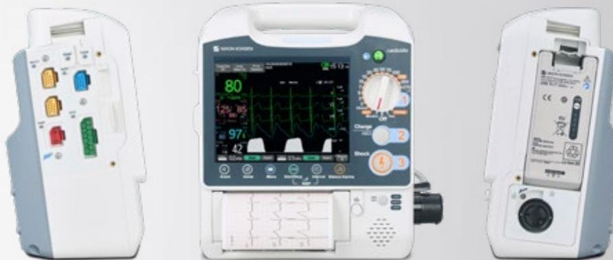
CardiolifeEMS is designed to fulfill the requirements of the demanding ambulance environment. With an IP55 rating and working on temperatures from -20 to 50 °C, it is suitable to use in almost all conditions out in the field. Thanks to its light weight of only 4.2 kg<sup>2</sup>, the rescue team won't have to worry about carrying another heavy device while rushing to the patient.
